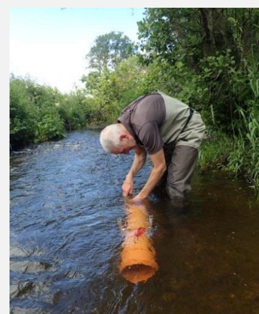
Figure 2 – Installing a sediment sampler on the Eddleston Water (left), a stream undergoing re-meandering as part of a NFM scheme coordinated by the Tweed Forum (right).
