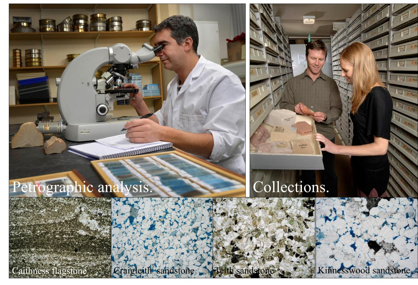
• Stone analysis and matching: petrographic techniques and our extensive collection of quarry samples and thin sections help us identify and source the closest-matching stone types to achieve a compatible, long lasting repair.
